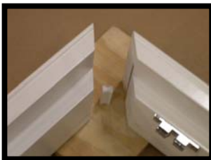
Set Hoffman Key Round side up and push top Frame down onto the Hoffman Key
